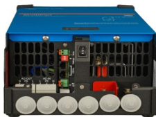
MultiPlus 2000 VA (bottom cover removed)
